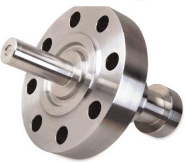
The PTX 400 series of pressure, temperature and combined pressure/temperature transmitters has been specifically designed for long term use in subsea locations. It enables accurate process measurements to be made directly on subsea wellheads and production manifolds. The sensor design is based on API performance requirement PRI and product specification level PSL3.
