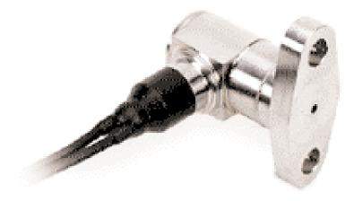
The PTX 300 series of pressure transmitters has been developed for the offshore oil and gas industries as a compact, high performance device for reliable and long term subsea use. Maintenance free, it is available with operating ranges up to 15,000 psi and is fully submersible with an ambient pressure rating up to 4000 psi.
